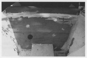
A new stern made of whiteoak was installed. Photo by Larry Ortt.
