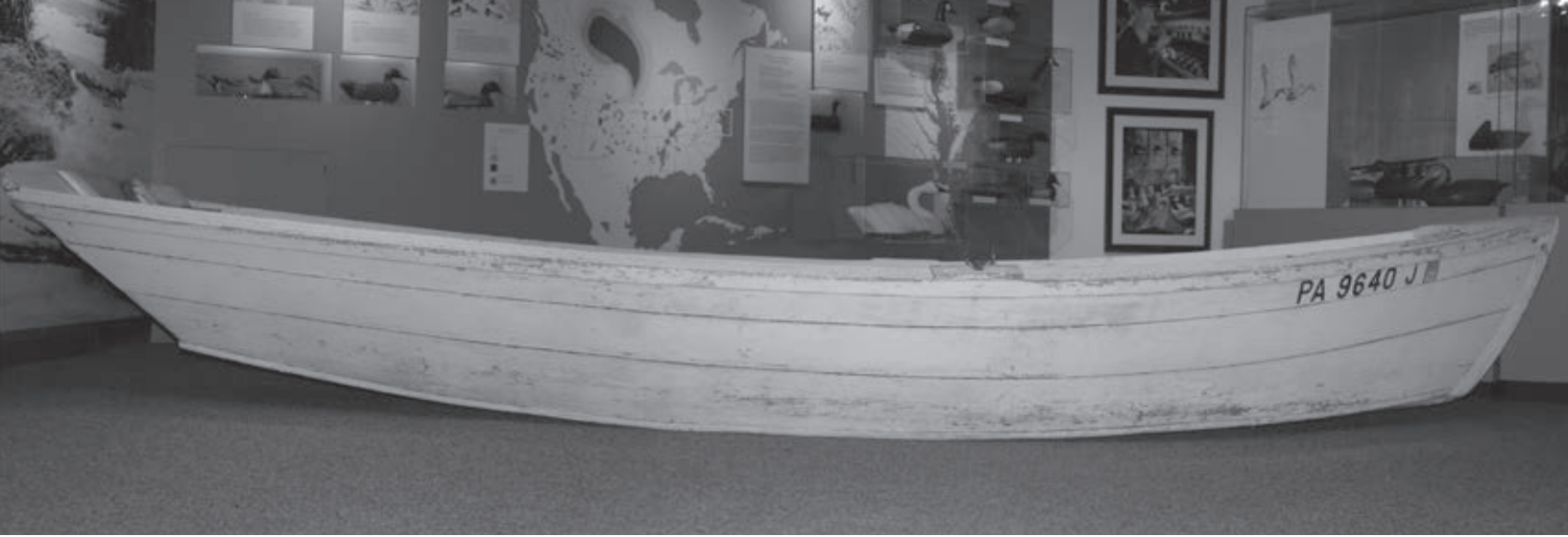
Thompson-built bushwhack boat at the Decoy Museum. Note that the bottom is convex with a fore and aft rocker and more rake to the bow and stern than other rowboats.
